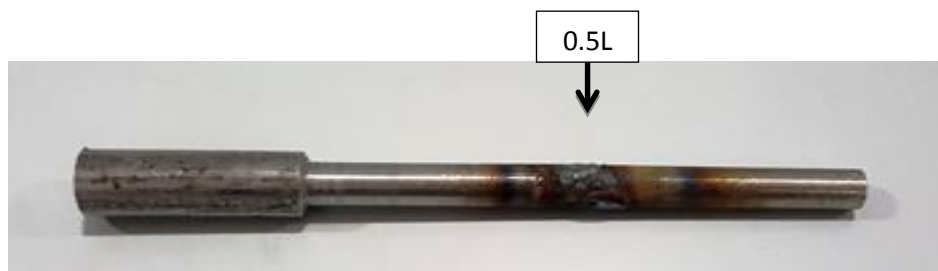
Figure 3. The weld is placed at a length of 0.5L from the shoulder.
