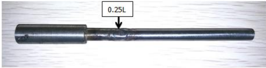
Figure 4. The weld is placed at a length of 0.25L from the shoulder.
