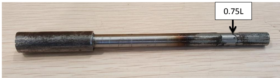
Figure 5. The weld is placed at a length of 0.75L from the shoulder.
